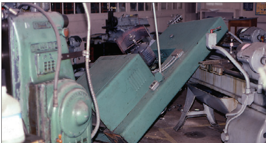
Figure 4-9: Fallen shop equipment, Coalinga, CA, 1983
