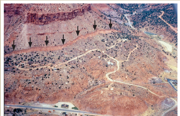
Aerial view of the Springdale landslide, triggered by the September 2, 1992, M 5.5 St. George earthquake. The top of the landslide is denoted by black arrows. Photo courtesy of the Utah Geological Survey.
