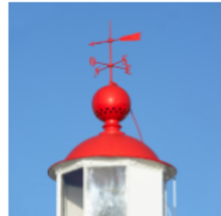
Weather Vane Measures wind direction
