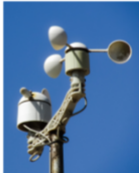
Anemometer Measures wind speed
