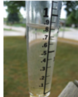
Rain Gauge Measures amount of precipitation
