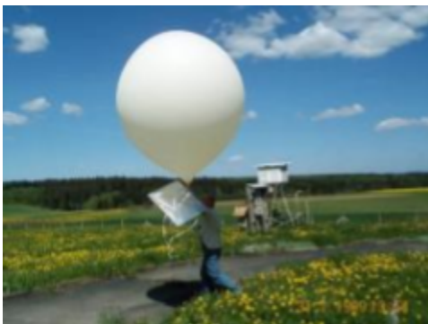
This weather balloon will rise into the atmosphere until it bursts. As it rises, it will gather weather data and send them to the surface.
